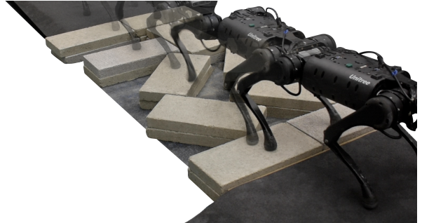
Fig. 1: The A1 quadruped robot walking over a random discrete terrain using our proposed approach. Video of experiments can be found here: https://youtu.be/3HAUvSsQYjs .
