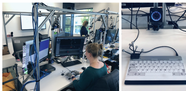
Figure 3. Our data collection setup consists of a marker-based hand-tracking system using OptiTrack cameras and a touchpad for recording contact. A printed 2D keyboard guide is attached to the touchpad for reference.
