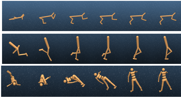
Figure 8. Noise to data paths computed with the trained CNFM on product manifolds representing robot’s state space: Cheetah (top), Walker (middle), and Humanoid (bottom).
