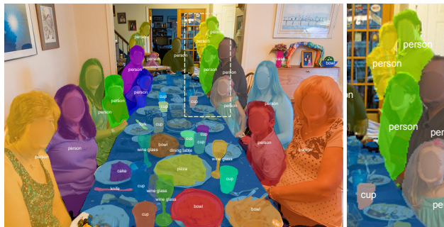
Figure 1. Selected output of TensorMask , our proposed framework for performing dense sliding-window instance segmentation . We treat dense instance segmentation as a prediction task over structured 4D tensors. In addition to obtaining competitive quantitative results, TensorMask achieves results that are qualitatively reasonable. Observe that both small and large objects are well delineated and more critically overlapping objects are properly handled .
