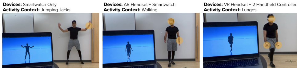
Figure 1: Using the activity context of jumping jacks, walking and lunges and inertial data from a smartwatch, smartwatch and AR headset and a consumer-grade VR headset and hand-held controllers respectively our system predicts the full-body pose.
