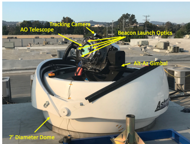
Figure 11: Rooftop dome assembly consisting of the AO telescope, the Alt-Az gimbal, and the beacon launch optics.
