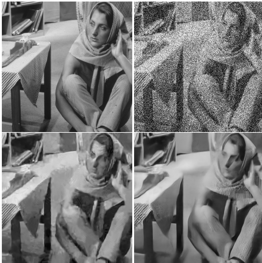
Figure 6: Visualization of denoising for the Barbara image with \sigma = 100 . Top-left is the original, top-right the noisy image, bottom-left is BM3D and bottom right is the output of a LBN. The LBN produces qualitatively more pleasing denoised images. There is a video of the distribution at http://ynd.github.io/lbn_denoising_demo/ .
