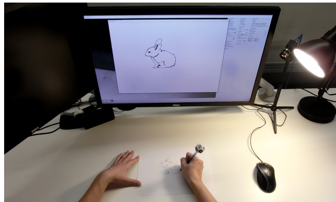
Figure 10. The DodecaPen can turn a flat surface into a digital drawing surface.
