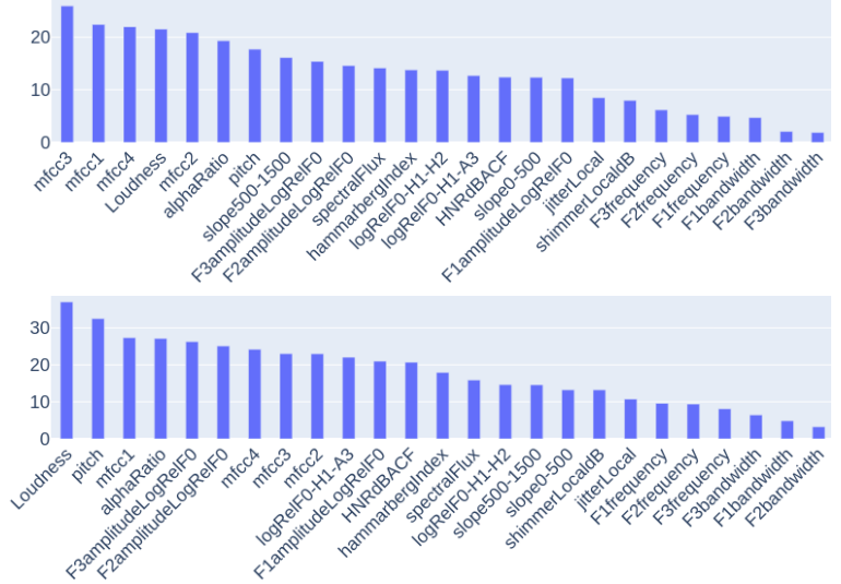
Fig. 1: Acoustic improvement (in %) for FullSubNet (upper) and Demucs (lower) by using the proposed PAAP Loss, where acoustic improvement is reduction in MAE as defined in Section 4.3.1.
