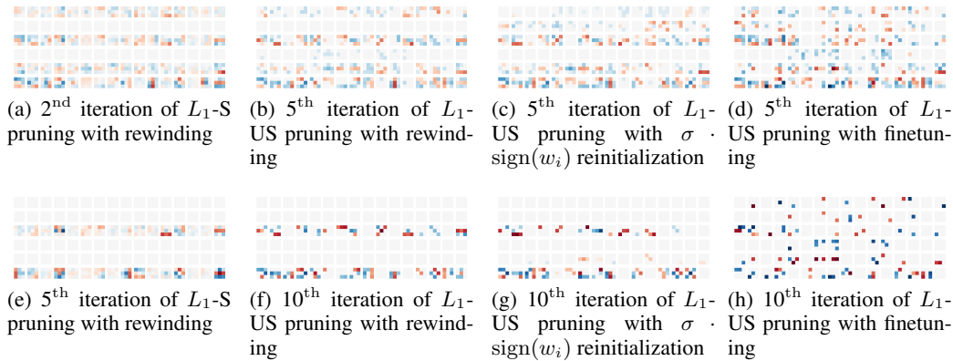
Figure 5: Masked weights in the 2 nd convolutional layer of LeNet. Rows represent two different pruning iterations. The columns represent four different pruning and weight treatments. The convolutional layer has 6 input channels and 16 output channels, with 3 \times 3 filters. Masked out weights appear in gray. Active, positive weights are depicted in red, negative weights in blue.
