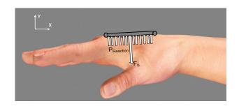
Fig. 3. Hand dorsum and simplified pHRI with uniform stiffness, bias force  $(F_b)$ , applied using straps and approximated as a point load at the center, and reaction pressure  $(P_{reaction})$ .
