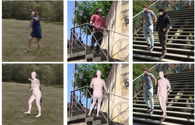
Figure 3: Typical failure cases of our method due to (left) body part occlusion, (middle) incorrect body orientation detection, (right) depth ambiguity of monocular camera.
