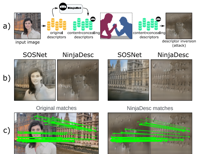
Figure 1. Our proposed content-concealing visual descriptor. a) We train NinjaNet , the content-concealing network via adversarial learning to give NinjaDesc . b) On the two examples shown, we compare inversions on SOSNet [75] descriptors vs. NinjaDesc (encoding SOSNet with NinjaNet). c) NinjaDesc is able to conceal facial features and landmark structures, while retaining correspondences. Image credits: laylamoran4battersea & sgermer (Flickr) 1 .
