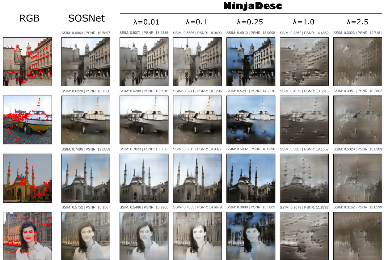
Figure 4. Qualitative results on landmark images. First column: original images overlaid with the 1000 (red) Harris corners [25]. Second column: reconstructions by the inversion model from raw SOSNet [75] descriptors extracted on those points. The last five columns show reconstruction from NinjaDesc with increasing privacy parameter \lambda . The SSIM and PSNR w.r.t. the original images are shown on top of each reconstruction. Best viewed digitally. Image credits: first 3 — Holidays dataset [29]; last — laylamoran4battersea (Flickr).
