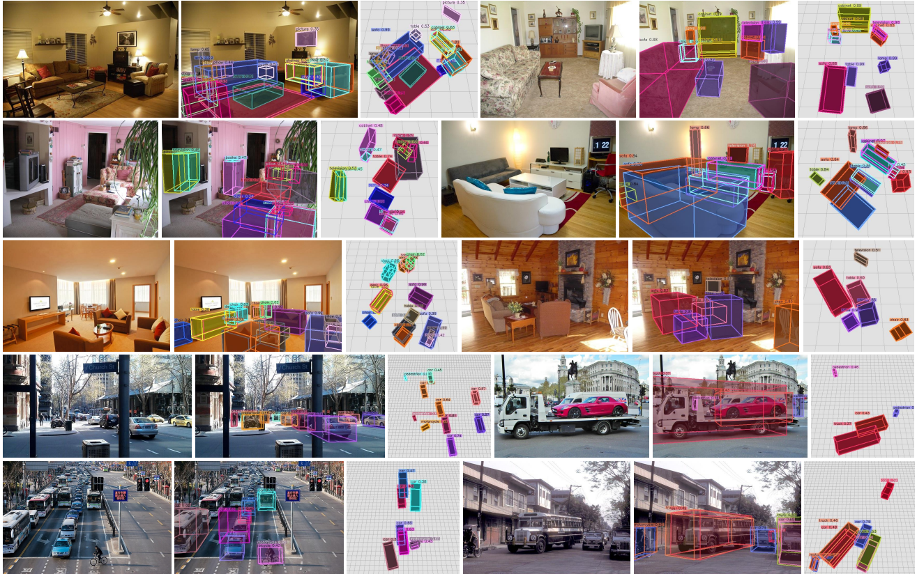
Figure 7. Cube R-CNN on COCO in the wild images. We select interesting scenes and observe that generalization performs well for indoor (Rows 1-3) compared to outdoor (Rows 4-5), which appear to fail when in the wild objects or cameras have high variation in unseen poses.
