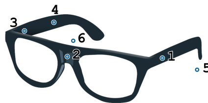
Fig. 2. Glasses microphone array used in EasyCom [12]. Mic 5 and 6 are in ears.
