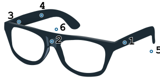
Figure 1. Illustration of the AR glasses with locations of microphones [4]. Four of the microphones are fixed rigidly to the glasses and two of the microphones are placed in the user's ears.
