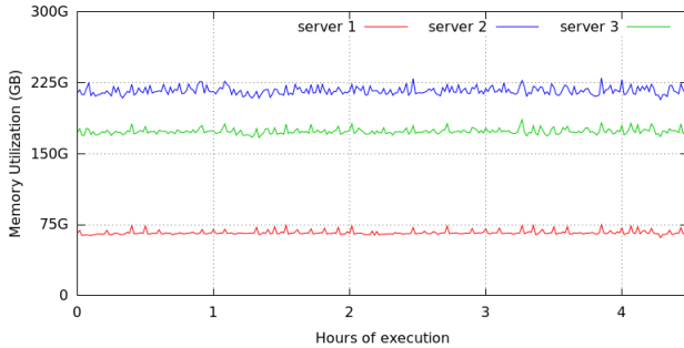
Figure 9: Memory utilization of servers ingesting data in real time with rollup enabled.
