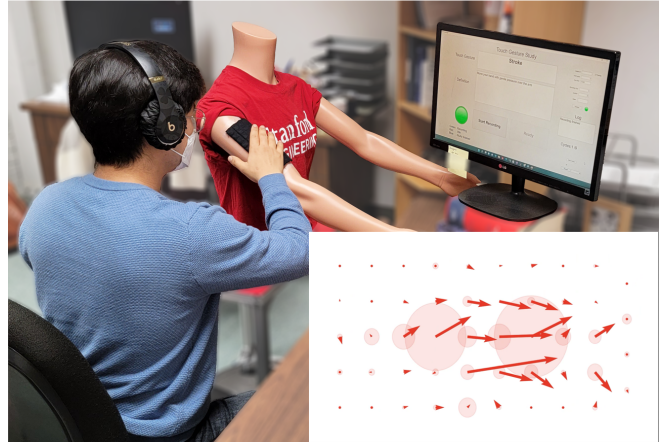
Fig. 1. User study setup for collecting touch gesture data consisting of a mannequin and our flexible sensing array. The bottom right plot shows sensor data; red circle diameters and arrows indicate normal and shear forces, respectively.
