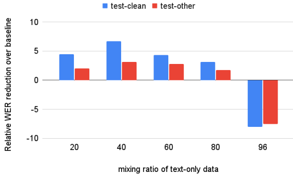
Figure 3: WER improvement of Rescorer with different mixing ratio on Librispeech.
