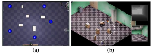
Fig. 3: (a) Top-down view of one of our testing environments. White boxes are obstacles. The robot navigates sequentially through the waypoints  $A \rightarrow B \rightarrow C \rightarrow D \rightarrow E \rightarrow A$ . Figure taken from [16]. (b) 3D visualization of the robot navigating in one of our testing environments in simulation. RGB and Depth observations are shown on the right.
