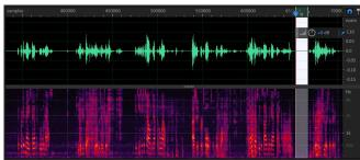
Figure 6(B): Waveform (top) and Spectrogram (bottom) after Our NS Processing.
