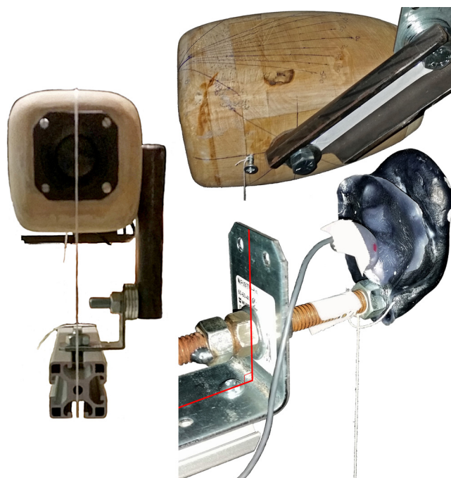
FIG. 1. (Color online) The used loudspeaker and the mounting of the pinna (lower right). The marked angle was verified to be 90^\circ (angle bracket used during first measurement session).
