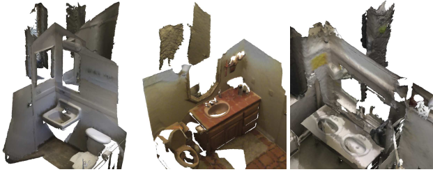
Fig. 2. Example scans from the ScanNet dataset [Dai et al. 2017] with artefacts due to mirrors.
