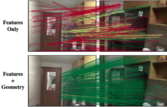
Figure 4. Geometry-aware sampling greatly improves our correspondence set. GART allows us to extract accurate correspondence even if the initial feature matches are very noisy.
