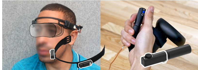
Figure 1. (left) A render of Chasm with a reference scale, the red arrow and wave represents how Chasm can simultaneously render both shear/normal forces and vibrations, (middle) A headgear prototype with two Chasm units on adjacent sides of the temple area on the head for enhancing locomotion in virtual reality (VR). A representative VR headset is shown. (right) A marker prototype with an embedded Chasm unit for enhancing interaction in augmented reality (AR) and virtual reality (VR), the hand is tracked with an attached Oculus Touch controller. The outlines show where Chasm is embedded in the prototypes.
