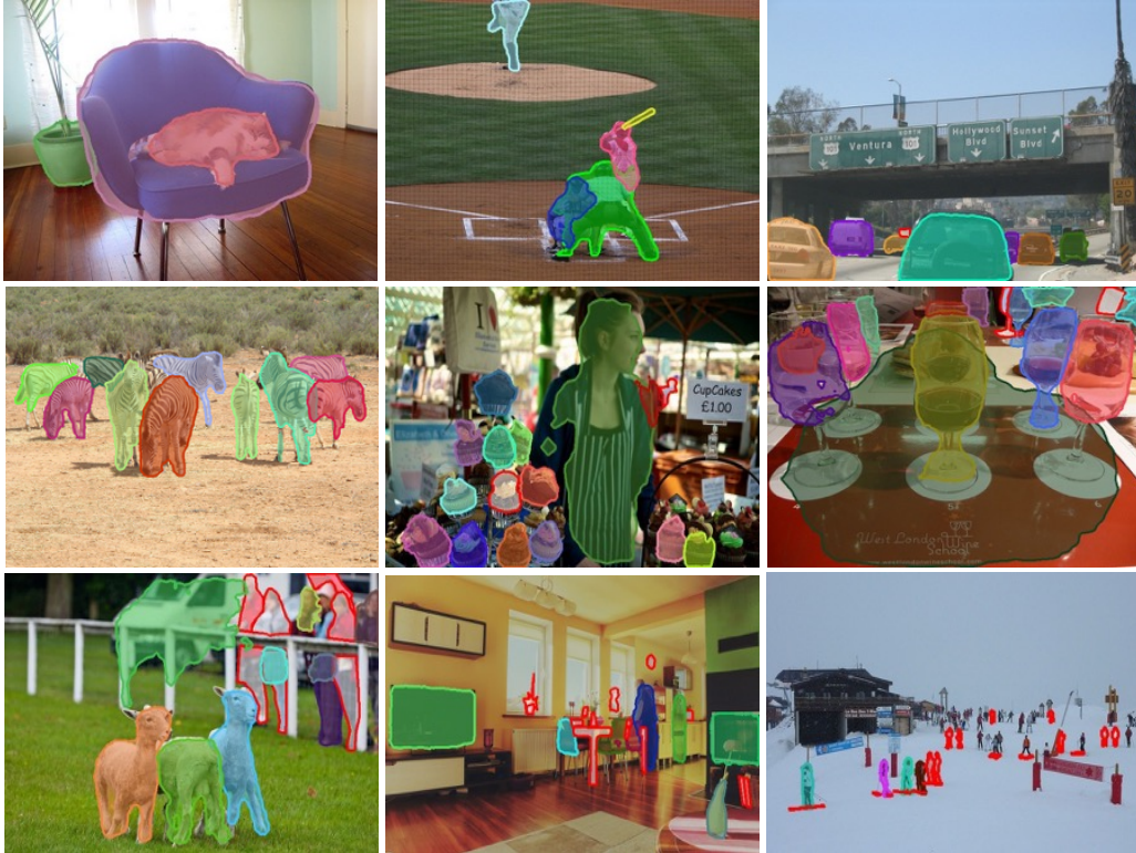
Figure 3: DeepMask proposals with highest IoU to the ground truth on selected images from COCO. Missed objects (no matching proposals with \text{IoU} > 0.5 ) are marked with a red outline.
