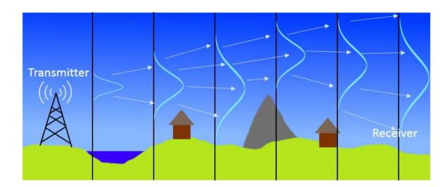
FFT is used to advance through each slice
