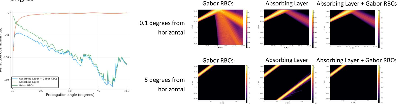
Reflection coefficient is computed by launching a beam at the upper boundary, letting energy reflect downwards or wrap around, and taking the ratio of final energy to initial energy
