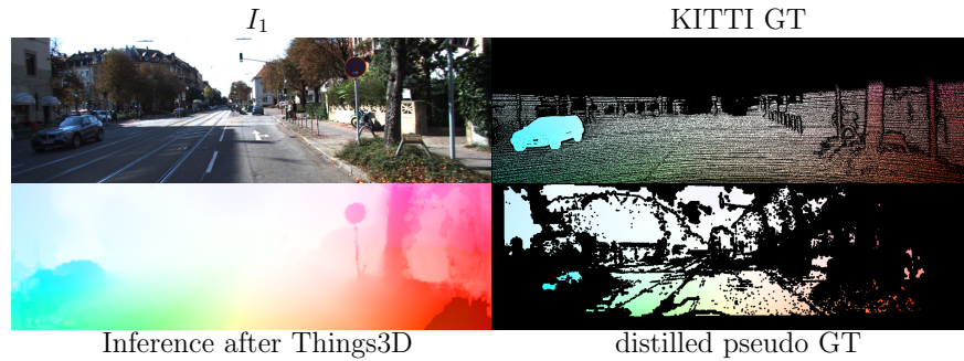
Fig. 6: Illustration of our data distillation process. Left to right: input image and associated KITTI ground truth, dense prediction from a Flying Things3D-trained network and pseudo-ground truth derived from it.
