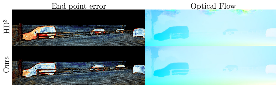
Fig. 3: Predicted optical flow and end point error on KITTI obtained with HD 3 from the model zoo (top) and our version (bottom). Note how our model is better able to preserve small details.
