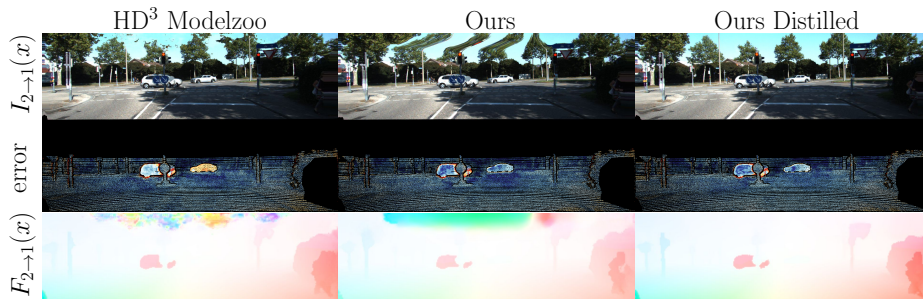
Fig. 7: Qualitative evaluation on KITTI, comparing the HD 3 modelzoo (left), our version with all contributions except distillation (center), and with distillation (right).
